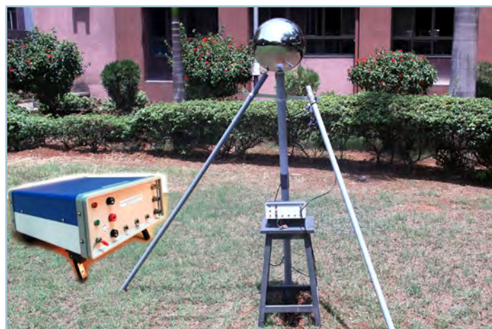
FIGURE 2 Schumann Resonance Receiver
